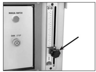
Figure 35. Blade stroke height lock knob.
